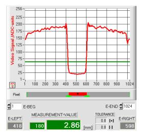
High video threshold, the object appears wider in the "shadow zone". Measured value = 180 pixel. The measured value in  $\mu$ m is calculated from this by multiplying the number of pixels with the respective pixel pitch.
