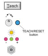
After a click on the TEACH button the current edge information is stored as a teach value to the RAM memory of the *L-LAS-TB sensor*. Depending on the evaluation mode that has been set (E-MODE), the left edge, the right edge, the width (WIDTH), or the center position (CENTER) will be stored as a teach value in the RAM memory of the L-LAS sensor.
