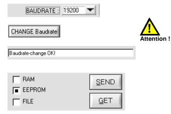
Baud rate setting at the sensor: Possible setting values are 9600Baud, 19200Baud, 38400Baud, 57600Baud or 115200 Baud.
