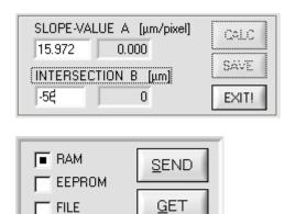
The calibration data also can be modified manually at the control unit of the sensor.
