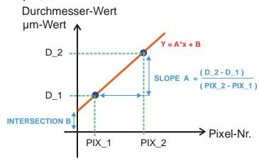
In two-point calibration, a mean straight line through two points is calculated on the basis of two known objects (dimensions in um are known) of different width.
