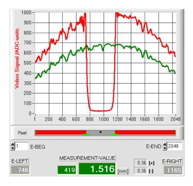
The y-axis shows the analog signals of the individual pixels. The analog values (video signals) of the CCD line are converted by means of an AD converter with 10-bit resolution, which results in a y-axis value range of 0 ... 1023.
