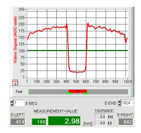
Low video threshold, the object appears somewhat narrower in the "shadow zone". Measured value = 188 pixel.
