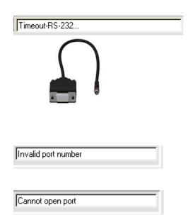
The serial connection between the PC and the *L-LAS-TB control unit* could not be established, or the connection is faulty.
